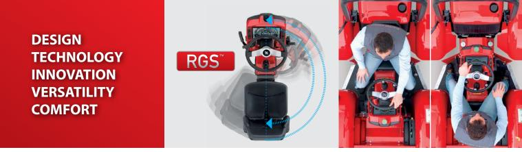
**TRX 7800"S"** isodiametric tractor with **Rev-Guide System RGS™**, the integrated system of technical solutions that allows you to rotate the driving position by 180° to use front tools such as fork lifts, arms, blades, shredders and snow blowers with ease. Its wide versatility of use makes this tractor suitable both for agriculture and civil maintenance at large sports centres, parks and public spaces, where it offers versatility in all seasonal activities.
